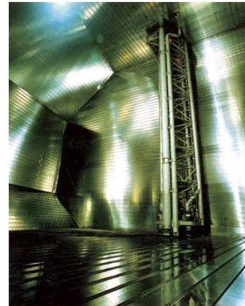
Membrane type LNGC and cargo tank
