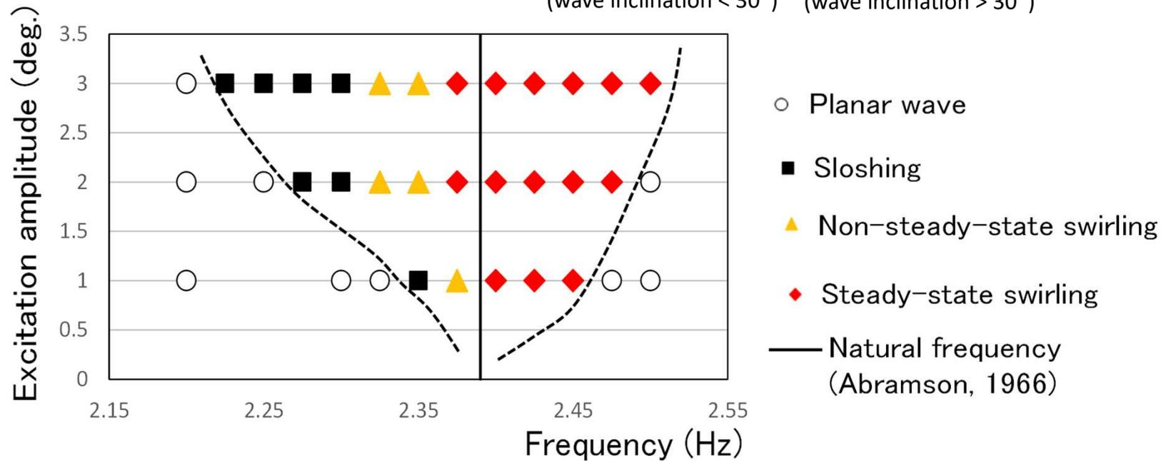
Behavior of the liquid motion in the spherical tank (filling ratio: 70%)
