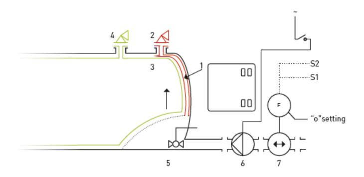
Excess air or an over-pressure underneath the inflated component can escape via a dedicated tube or hose "3" and relief valve "2".
