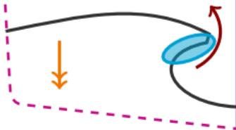
$$\underbrace{\frac{1}{1 + \mathcal{R}_\rho}}_{\approx 1} \underbrace{\left( \frac{\text{inertia}}{\text{surface tension}} \right)}_{\text{Weber number}} + \underbrace{\left( \frac{\text{gravity}}{\text{surface tension}} \right)}_{\text{Bond number}} > 1$$
