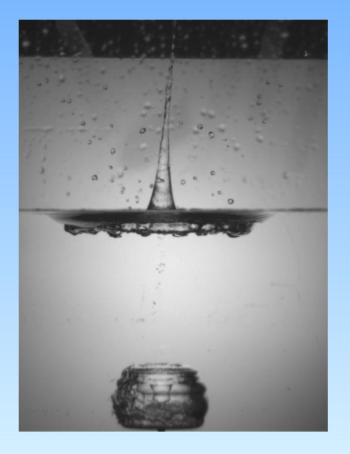
void creation void collapse jet creation at singularity air-entrainment "giant bubble"
